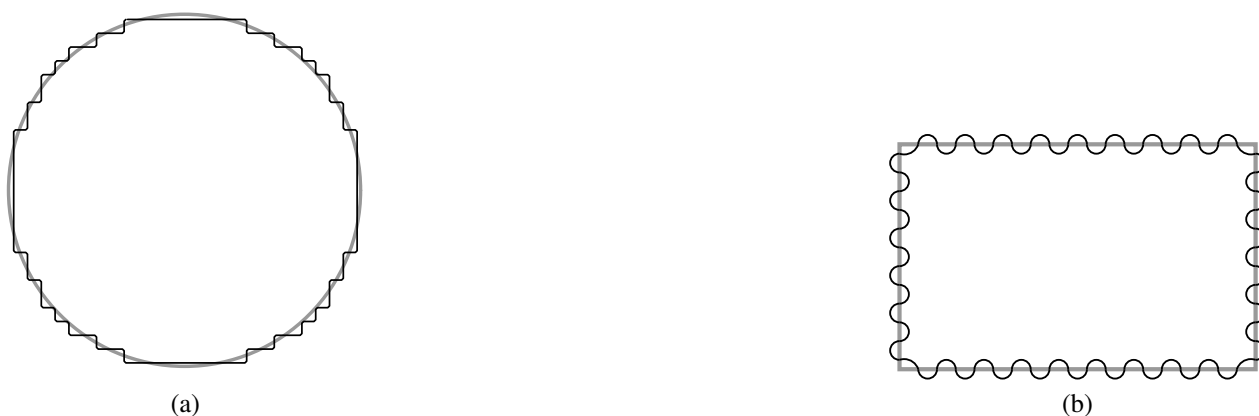
Figure 5: Two shapes (in gray) with local modifications (in black) causing a reversal in measured rectilinearity. a) The circle is quantised on a square grid. b) The rectangle has a series of semi-circles superimposed.
