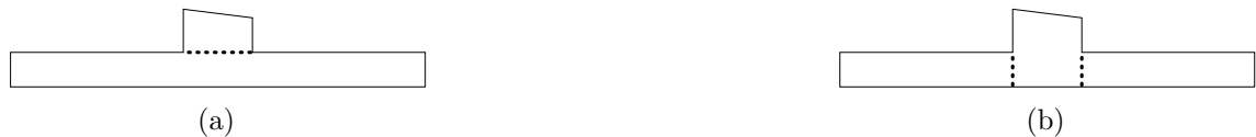
Figure 6: Should cuts be made to (a) the closest negative curvature minimum (b) the closest boundary point irrespective of its curvature?
