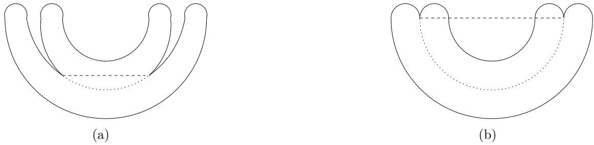
Figure 4: The requirement for curved part boundaries; (a) a curved cut is more appropriate than a straight cut, (b) only the curved cut is valid.
