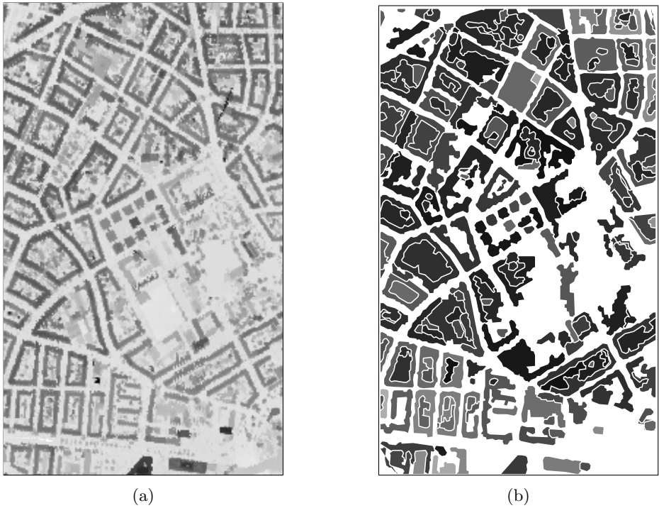
Fig. 7. (a) A DEM of Hannover; (b) segmented regions with filled intensities proportional to rectilinearity
