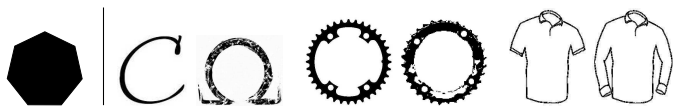
Fig. 13. The reference polygon \mathbf{P} is selected to be a regular 7-gon (on the left). The remaining shapes have IoU_{\mathbf{P}}(S) value equal to 0. Their \mathcal{G}_{\mathbf{P}}(S) values vary, and they are: 0.3088, 0.4024, 0.4408, 0.4631, 0.2443, and 0.2667, respectively.
