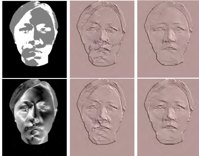
Figure 16: Alternative surface combination methods. Top: 0–1 combination map, relief from 0–1 map, relief using default averaging approach. Bottom: Weighted combination map, relief from weighted map, relief using weighted map to produce normals and integrating.
