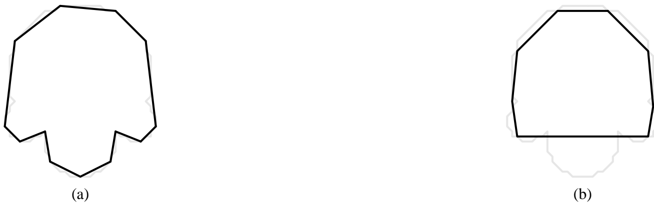
Fig. 6. Some approximations of figure 4; (a) Result of Lowe's algorithm, (b) Result of Sankar & Sharma's algorithm
