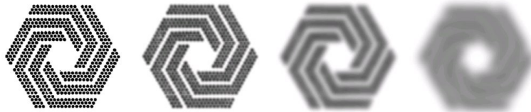
Fig 2. The four levels of Gaussian smoothing applied to a complex image
