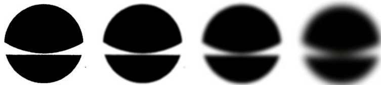
Fig 1. The four levels of Gaussian smoothing 0-3 derived from a simple image. Level 0 (left) is the original image.
