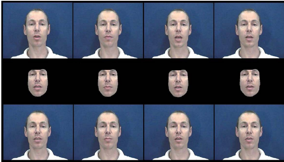
Figure 7: Background registration of facial images generated by our synthesis algorithm: Background images taken from the training set (Top), and facial images generated from our synthesis algorithm (Middle), are aligned and merged to produce output frames (Bottom).
