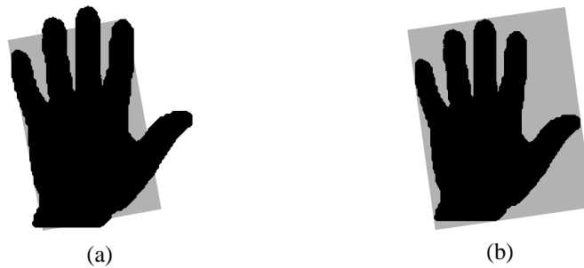
Fig. 12.6 The rectangle shown in (a) was fitted according to (12.7) as compared to the minimum bounding rectangle shown in (b).
