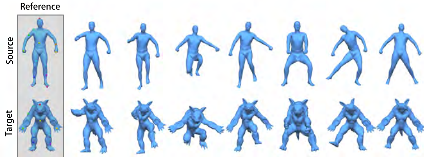
Figure 5: Results of transferring the deformation on the source mesh (a human from the SCAPE dataset) onto a different target mesh (the Armadillo model) using our method with automatic key point selection. Correspondences are highlighted using colored balls where the same color indicates corresponding points. The first column contains the source and target meshes without deformation. The first row shows the source meshes and the second row gives the output meshes. The deformations of input meshes are reproduced successfully on the target mesh, even with substantial geometric difference and large deformations.
