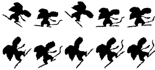
Fig. 12 Normalised data with a 1.1 scale factor in X and added noise; upper row orientated using moments, lower row orientated using squareness ( \beta = 8 ).
