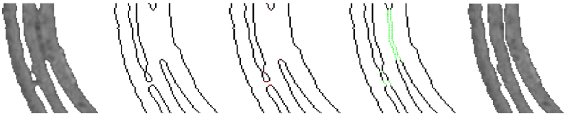
Figure 6: From left to right: segmented parchment fragment; its contour; endpoints detection (red); links construction (green); postprocessed fragment
