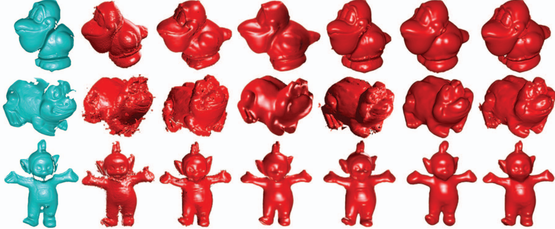
Figure 1. Rows: Reconstructions using 17 Bird range images, 17 Frog range images and 17 Teletubby range images respectively. From left to right: one single range image used as partial ground truth, volumetric method [3], mesh-based method [15], SFK method [20], k-means clustering-based method [19], pairwise MRF-based method [11], higher-order CRF-based method [14]
