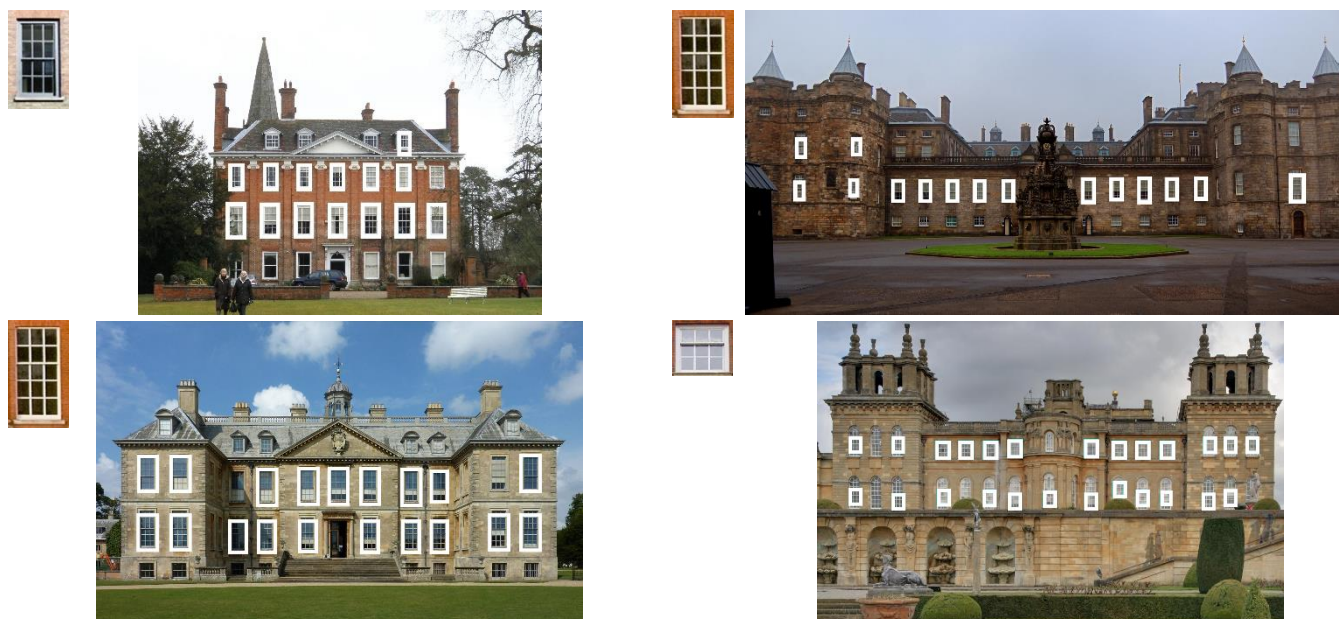
Fig. 3 HOG-based template matching over varying scales on Flickr images of UK heritage properties Welford Park 3 ( top-left ) and Holyrood Palace 4 ( top-right ), a Wikipedia image of Belton House 5 ( bottom-left ) and a Flickr image of Blenheim Palace 6 ( bottom-right ). For each image the template used is shown top-left, with matches as thick white bounding boxes .
