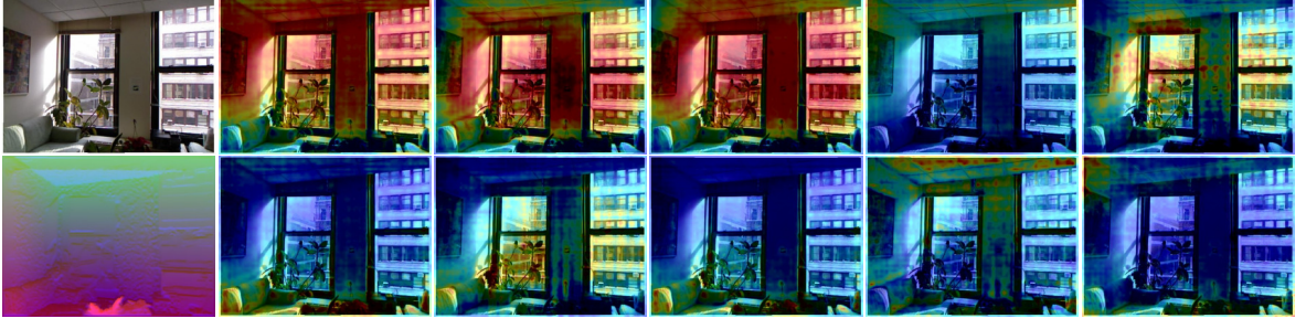
Figure 3: Illustration of the scale-aware confidence map. The two images in the first column are RGB and depth images. The two images in the second column are scale-aware confidence maps upon the two modalities. The remaining 4 images in the first row are each scale channel confidence map of RGB modality, in the second row are each channel confidence map of depth modality. From left to right, they are a_6 , a_{12} , a_{18} , a_{24} . For the sake of simplicity, we show the confidence maps (average value) by using the “COLORMAP_JET” color map (where blue is low value and red is high value) upon RGB. Best viewed in color.
