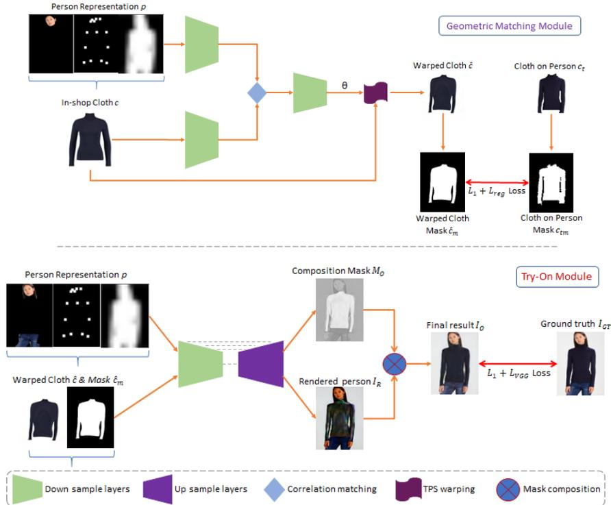
Figure 2. Full pipeline of our proposed CP-VTON+.
