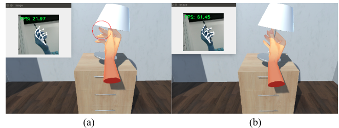
Fig. 1. A simple game interaction scene. (a) A scene in which the linear blend skinning model of the hand is driven by the predicted 3D joint points of the hand in the video to interact with the object at low FPS. (b) Interactive scene at high FPS. At low FPS, there is a possibility that the prediction of the 3D joint points of the hand in a certain frame is inaccurate, resulting in abnormal hand deformation when driving the linear blend skinning model of the hand, as highlighted by the example in the red circle where the finger deforms abnormally. Best viewed in color.
