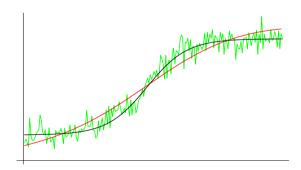
Too Little Training: This shows the performance of a neural network at the beginning of training. The training data is shown in green. The data was created by adding a measured amount of noise to a logistic curve. The original curve is shown in blue, so that is what we are trying to model. The predictions of the neural net are shown in red. After a few rounds of training, the network has got the general shape, but it hasn't yet modeled the curve very accurately.
