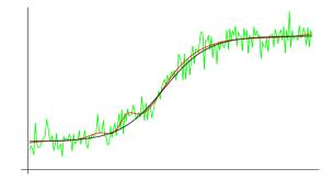
Too Much Training: This shows the performance of a neural network that has been overtrained. As the network is adjusted to fit the data, it begins to fit the noise rather than the underlying function.
