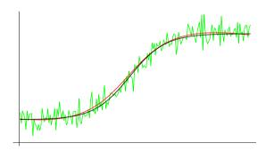
Just Right Training: This shows the performance of an optimally trained neural net. The original underlying function has been modeled almost exactly. **This is** the model we want to build. This model was built by training the network until its error was equal to the noise estimate provided by the Gamma Test
