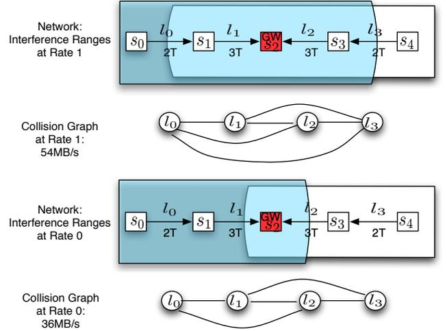
Figure 7: Network for example showing the benefit of multiple rates.
