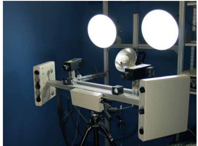
Fig. 1. Photographic representation of the 3dMDFace™ Dynamic System taken with Fujifilm F31fd digital camera.
