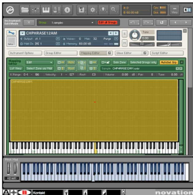
(Single key mapped) Single Velocity Layer — Only **one** type of sound played at **any** **velocity**.
