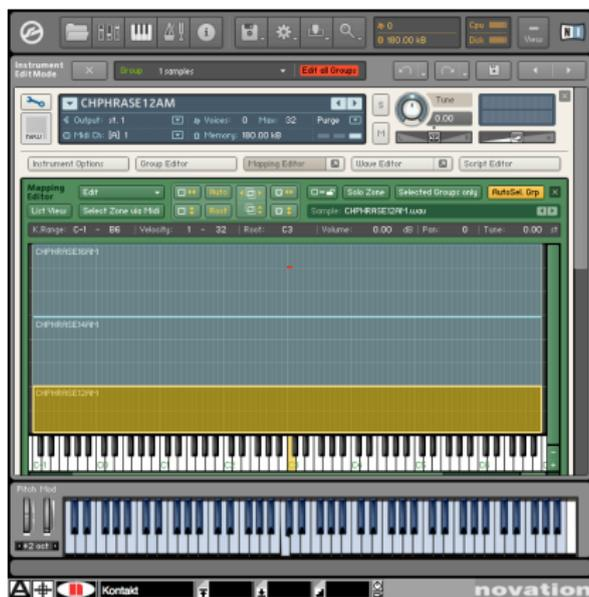
(Single key mapped) Triple Velocity Layer — Three type of sounds played according to velocity.
