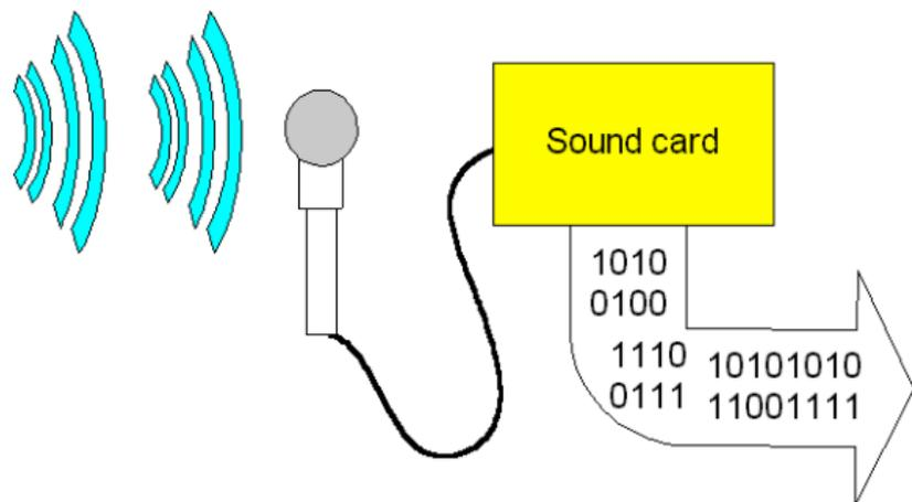
Take analog signals from analog sensor (e.g. microphone) and digitally sample data
