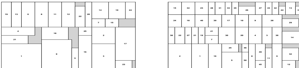
Figure 3: GA packings for 25 and 50 rectangle problems from [6]: width = 40, height = 16
