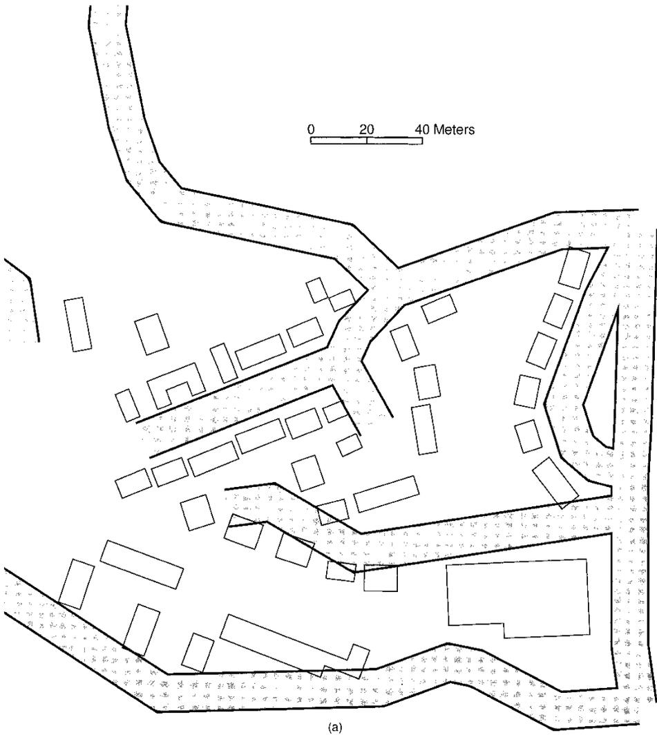
Figure 10(a). Large scale OS data example. (a) Graphic conflict arising due to scale reduction and road symbolization.
