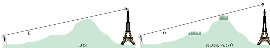
**Figure 1** Determination of whether a surface profile is line-of-sight (LOS) or non line-of-sight (NLOS)
