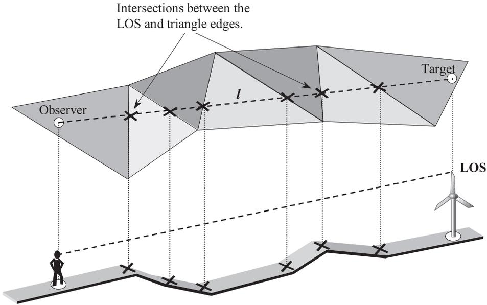
**Figure 2** Re-construction of a surface profile ( $l$ ) through a TIN with linear interpolation across the triangle edges
