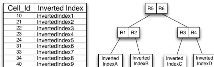
**Figure 5.4:** Spatial first spatio-textual indexing with a quadtree (left) and an R-tree (right). Note that the inverted indexes referenced by the nodes of these structures refer just to those documents whose footprints intersect that node. Data must also be stored for each document footprint so that it can be tested against the query footprint.
