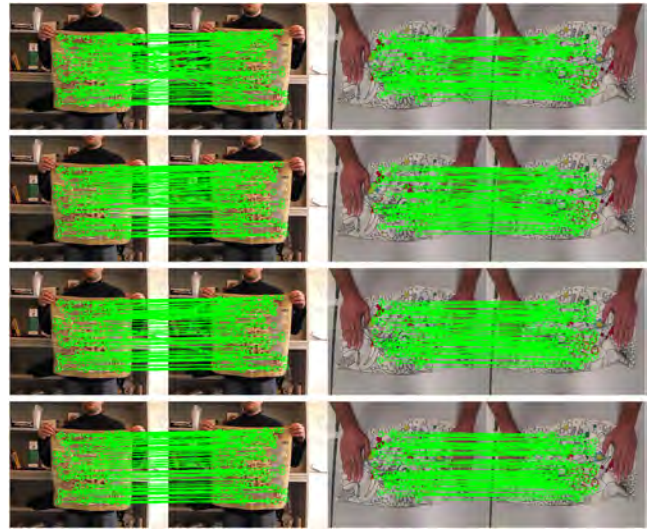
Fig. 8. Matching results. Left: cloth set, matching between frame 80 and 90, right: cushion set, matching between 144 and 156. Top to bottom, spectral method [26], hypergraph matching method [28], a third-order tensor method [21], [29], and SuperMatching.
