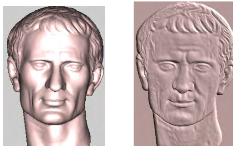
Figure 2: Two images rendered under the same conditions: a 3D model, and a bas-relief generated from it using the method in [5]. Note that these images are very different.
