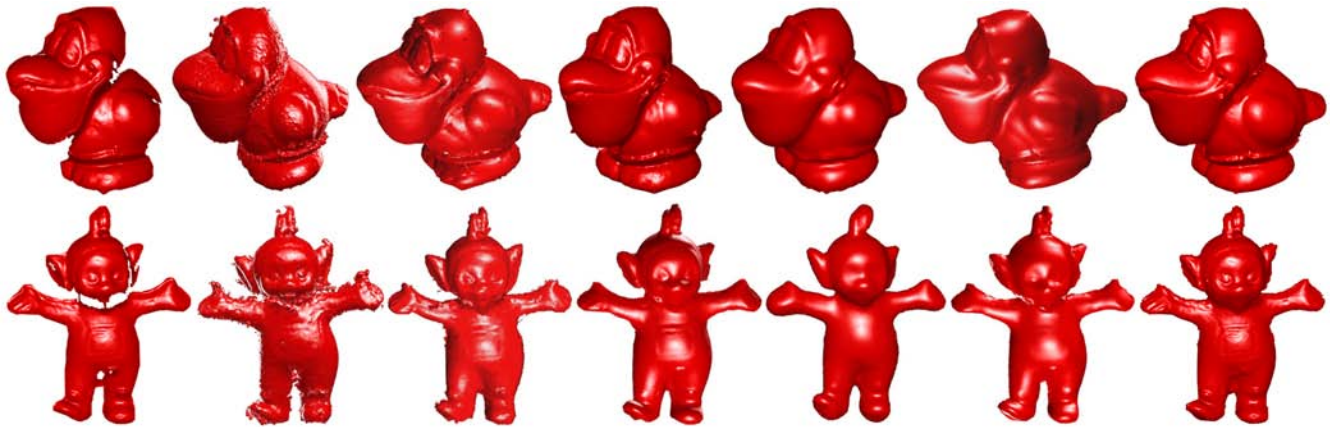
Figure 5. Rows: Integration results of Bird and Teletubby scans. From left to right: one input scan (ground truth), volumetric method [8], mesh-based method [22], k -means clustering [25], pairwise MRF [16], SFK [26], our method
