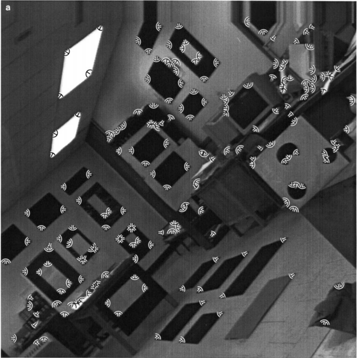
FIG. 13. Corner properties measured from real image. (a) Orientation and angle; (b) contrast; (c) bluntness.
